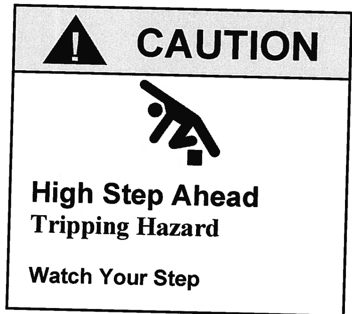
FIGURE 53.4. Example of a sign warning against a trip hazard.
