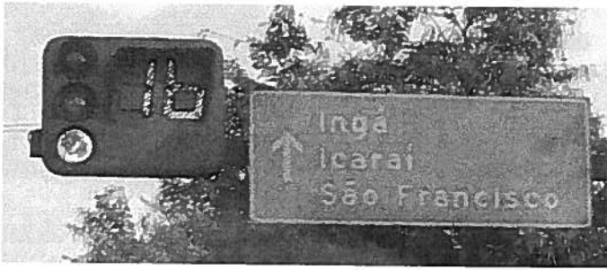
FIGURE 63.2. A traffic signal countdown sign. (See Color Plate 22).
