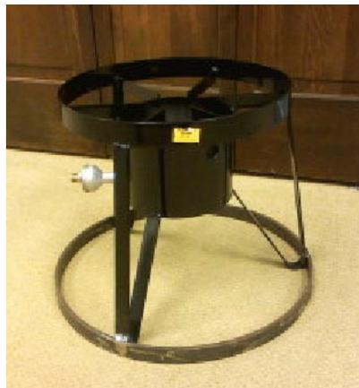
A significant hazard associated with this product is that it is unstable and can tip over if intentionally or unintentionally bumped or moved. The resulting hot oil spill can result in severe or catastrophic burns. Such incidents have occurred in situations such as outdoor picnics or similar events where children or animals may be active in the vicinity of the cooker.
