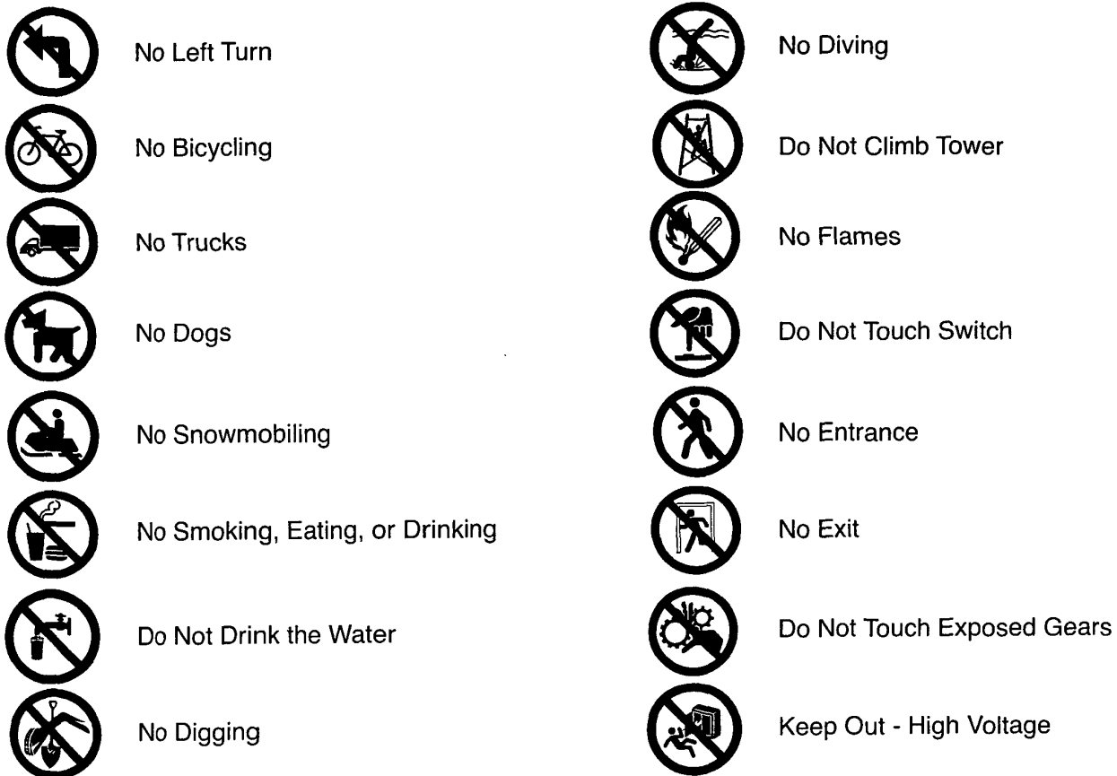
Figure 1. The 16 base pictorials used in the experiment. The circle slash component was in red; the base pictorial symbol was in black
