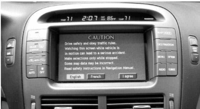
**Figure 8.9.** In-vehicle navigation system displaying a warning.
