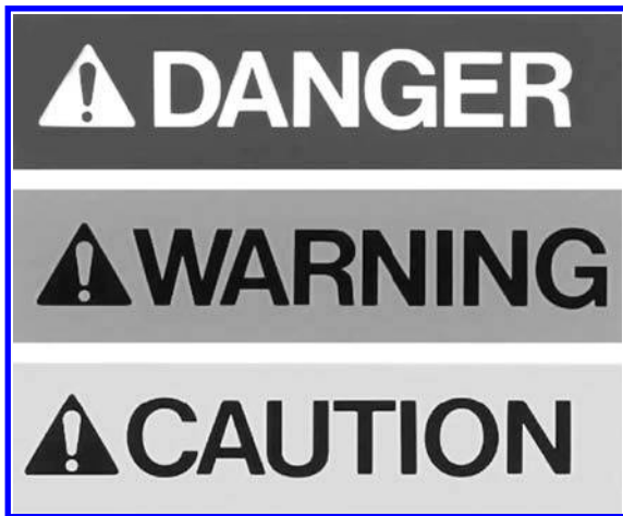
FIGURE 2 ANSI Z535 signal word panels. The colors tied to DANGER, WARNING, and CAUTION are red, orange, and yellow, respectively.
