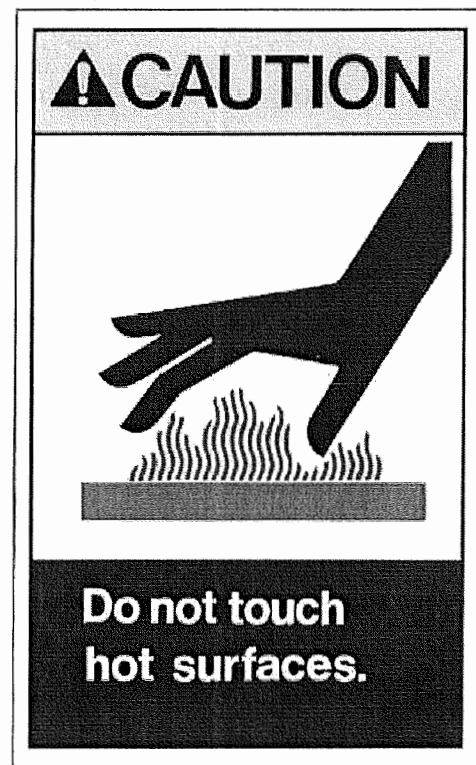
FIGURE 12.14. ANSI-type warning sign that has red color to highlight the radiant heat. (See Color Plate 4).
