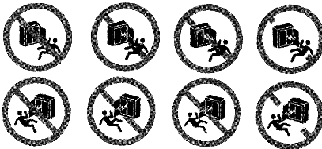
Figure 2. Example Pictorial in the 8 Variations of Slash Type (Over, Under, Partial and Translucent) and Orientation (Left-I and Right-II).
